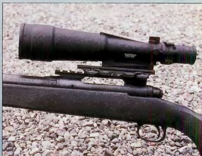
As with all optics tested, the TA55 ACOG was mounted on a Ross Optical Platform using A.R.M.S. ThrowLever mounts.
